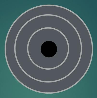
Each surface is divided into rings called <u>tracks</u>. A stack of tracks (across platters) is called a <u>cylinder</u>.
