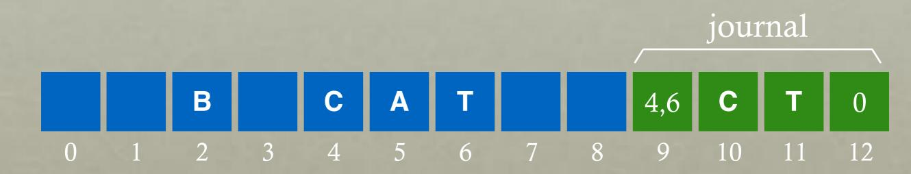
transaction: write C to block 4; write T to block 6 write order: 9, 10, 11, 12, 4, 6, 12
