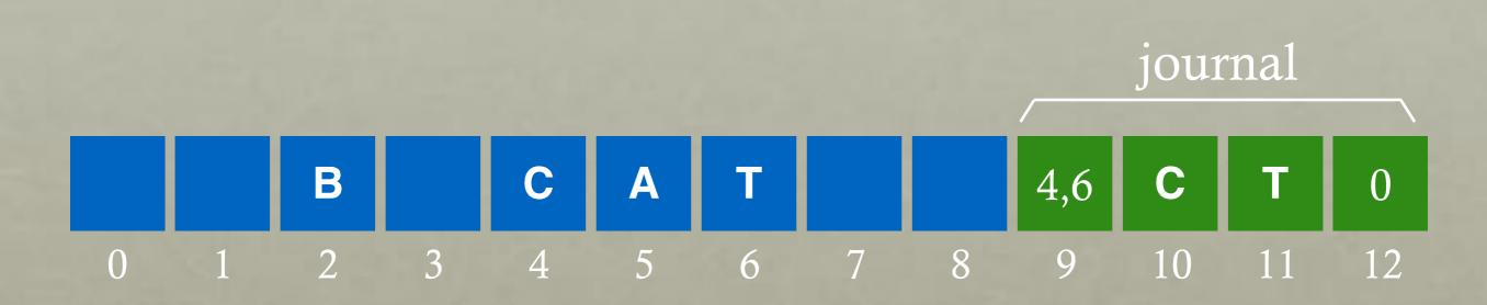
transaction: write C to block 4; write T to block 6 write order: 9,10,11 12 4,6 12
