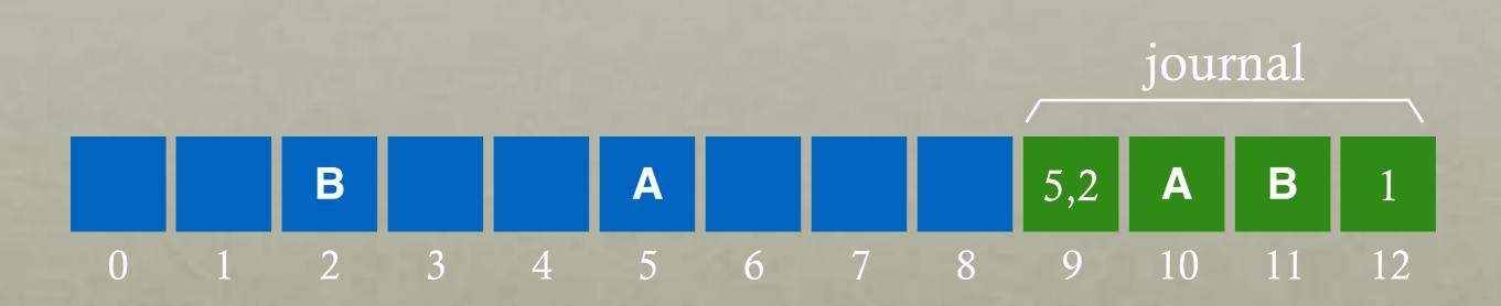
transaction: write A to block 5; write B to block 2
