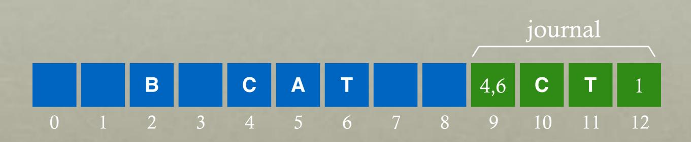
transaction: write C to block 4; write T to block 6
